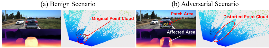
Fig. 1: Attack MDE and 3D object detection with a natural adversarial patch. The left is a benign scenario and the right is the corresponding adversarial scenario. 3D object detection takes the pseudo-Lidar ( i.e. , point cloud projected from 2D depth map) as input and outputs bounding boxes of recognized objects. Observe in the adversarial scenario (b) that our optimized adversarial patch can disturb the depth estimation of the target vehicle significantly and the effect propagates to an area larger than the patch itself. Pseudo-Lidar of the vehicle is thus distorted and it cannot be detected in the downstream task.
